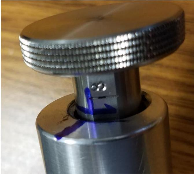
Once properly adjusted, mark the adjustment screw so readjustment can be easily duplicated by turning the screw. This can be accomplished with a permanent marker or with tape and a pen. When checking multiple buttons, it is quite possible to bump and turn the adjustment screw without knowing it. Markings will ensure the gauge stays properly set and will allow for resetting if needed.
